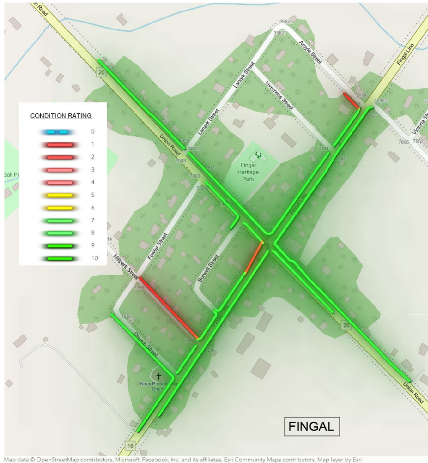
Figure 5: Fingal Sidewalk Condition Rating Map
