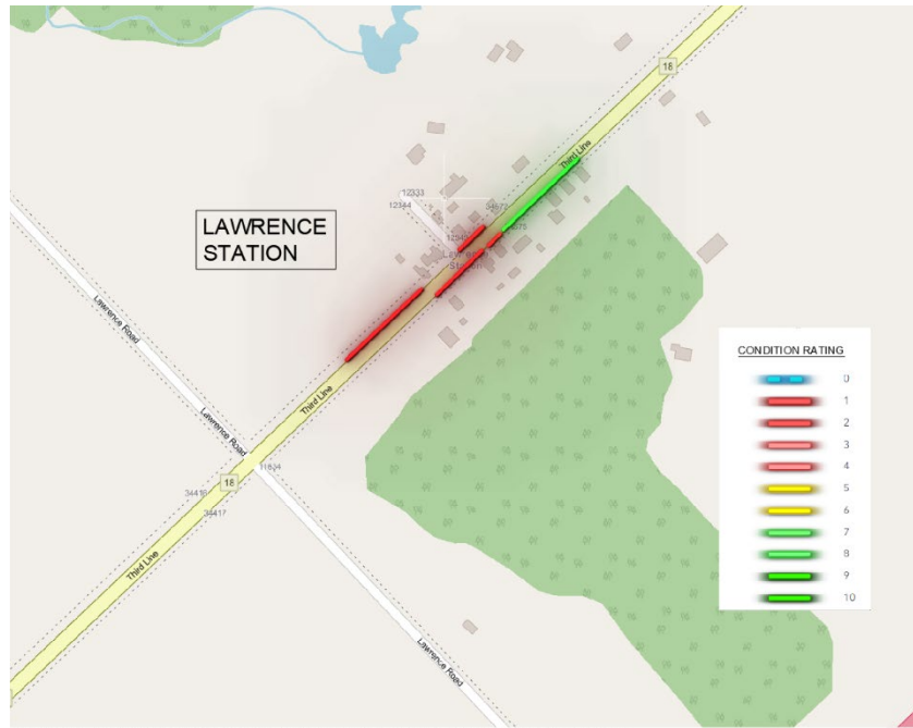
Figure 1: Lawrence Station Sidewalk Condition Rating Map
