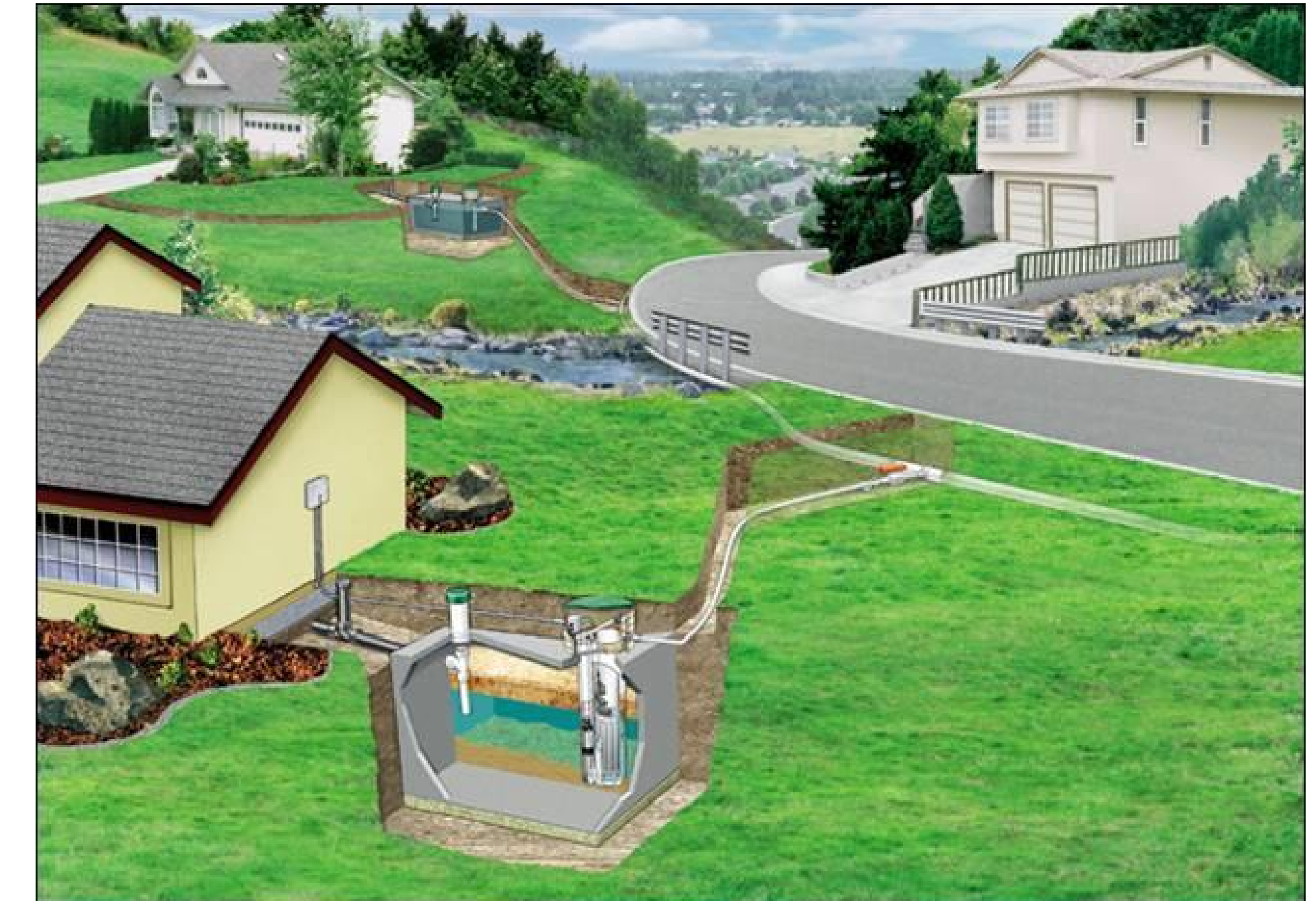
Example of a STEP Low Pressure Sewer
