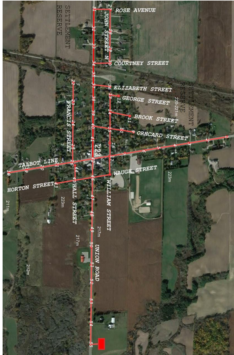
Figure 3: Potential Shedden Collection System
