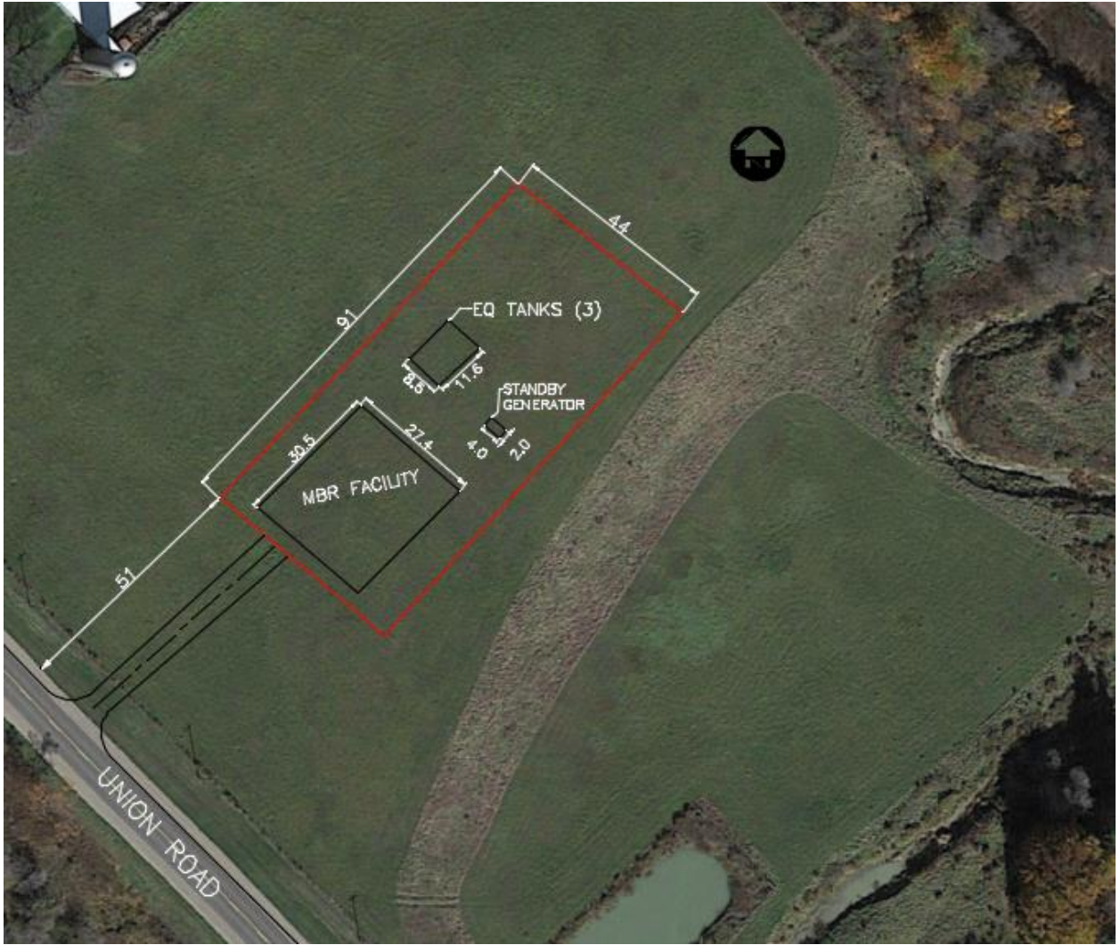
Figure 2-5: Shedden Location – MBR Facility
