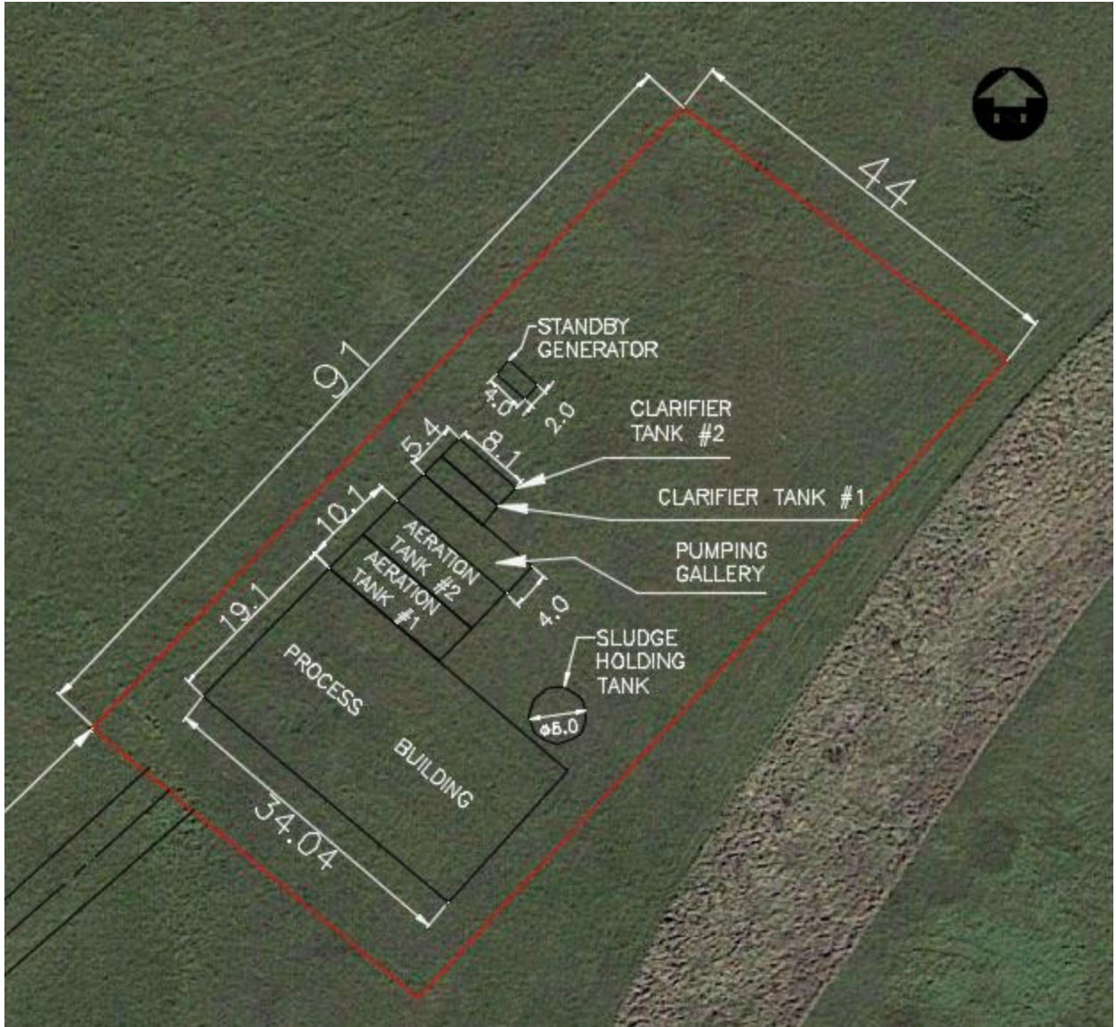
Figure 2-2: Shedden Location – Extended Aeration Facility Detail
