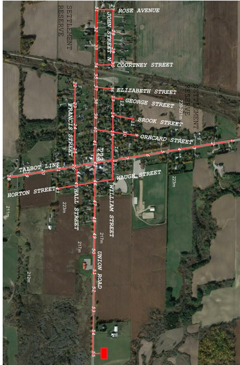
Figure 3-2: Potential Shedden Collection System
