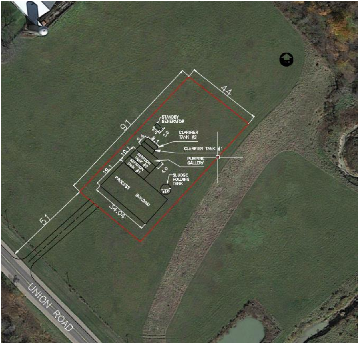
Figure 2-1: Shedden Location – Extended Aeration Facility
