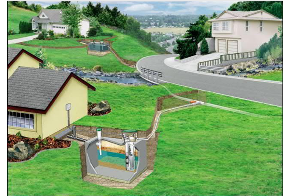
Example of a STEP Low Pressure Sewer
