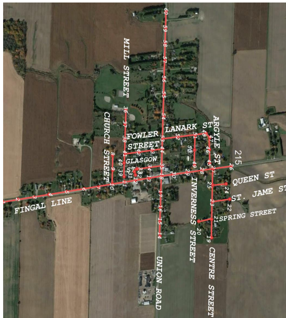
Figure 3-1: Potential Fingal Collection System
